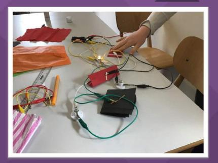
Using their knowledge of electrical circuits, children in Holly Class worked in groups to design and build a set of working traffic lights. The challenge was to make a circuit which they could control to ensure only one light came on at a time.
