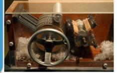
machine that quickly and easily separates cotton fibres from their seeds.
