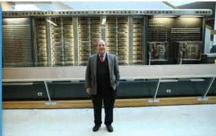
in 1945 a patent for the Automatic Sequence Control Calculator was filed. The Mark I (as it was known) was a large automatic digital computer that could perform the four basic arithmetic functions and handle 23 decimal places. A multiplication took about five seconds.
